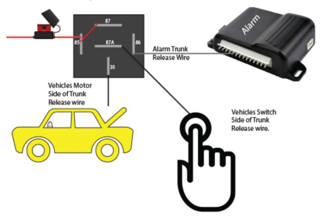
Using a standard 30 Amp automotive SPDT (single poll double throw) relay you will be able to convert a negative output from your alarm or remote start into a positive output. You can also create a stronger negative trunk output by triggering a relay. On vehicles that require reverse polarity to release the trunk, this can be accomplished using the standard 30 Amp SPDT relay. Follow the diagrams for the system that will work for your install.
